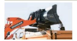
With a sloped bottom for maximum filling and material retention, this is the perfect bucket for day-to-day material handling. Capacities range from 4 to 6.5 yd<sup>3</sup>.
