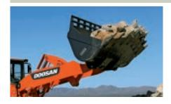
Severe digging is no problem for this tough bucket. Spade nose style. Weld-on teeth come standard. Capacities from 4 to 6 yd<sup>3</sup>.
